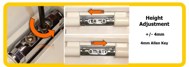
Lateral Adjustment: (Note Lateral and height adjustment can be made simultaneously) Slacken off both M5 Cap Head Screws **on all hinges** (and ensure they are re tightened after adjustment) The Door can now be moved up or down about the nominal position
