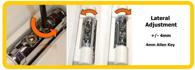
Lateral Adjustment: (Note Lateral and height adjustment can be made simultaneously) Slacken off both M5 Cap Head Screws **on all hinges** (and ensure they are re tightened after adjustment) The Door can now be moved one way or the other about the nominal position
